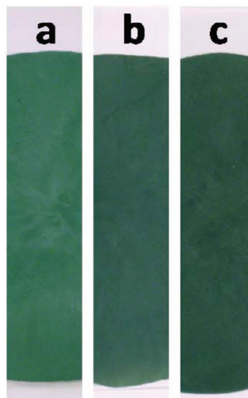
Figure 2. Photographs of 100 μm thick hot-pressed films of green-to-colorless TCM-PP composites with different TCM contents. (a) 10 wt %; (b) 15 wt %; (c) 20 wt %.
