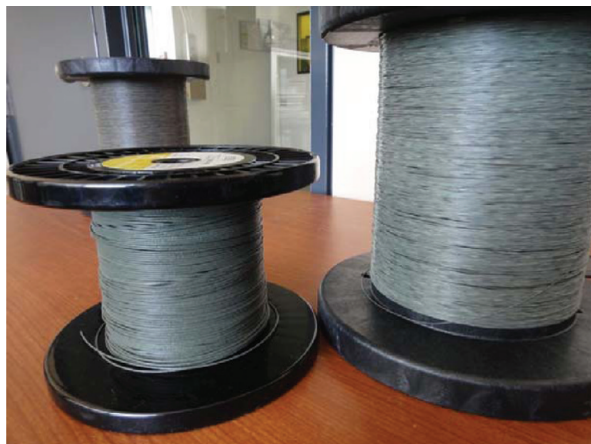
Figure 4. Spools of a green-to-beige trilayer coaxial monofilament after melt-spinning (left) and after solid-state poststretching at a ratio \lambda = 7 (right).
